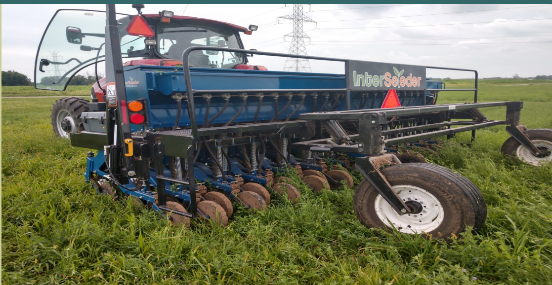
Ozaukee County InterSeeder used as no-till drill into cover crop mix. Photo taken August 12, 2019.
